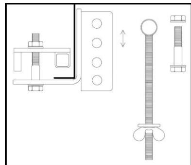
For optimum and safe functioning (properly clamp securing the spare wheel), it is important that there is 10mm space (A) between the chassis mounting clamp bolt and the bracket. If necessary, fill the space between the wheel and the caravan bottom with a wooden bar.
