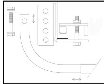
Determine the final position of the spare wheel and secure thereafter the transverse bracket with the M10x85 threaded pin (turn into the welded nut). Lock the threaded pin then with the M10 nut so it will not come loose.
