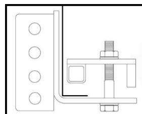
Mount the chassis clamp plates on the right chassis side (*passenger side*). Use again the M10x60 bolt, 2 M10 washers, M10 locking nut and fix it "by hand", so much so that the chassis mounting clamp can be just shifted.
