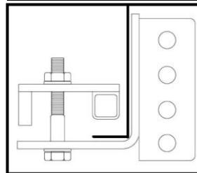
Slide the transverse bracket (C), with the welded-on nut upwards, over the thicker tube (B) of the Telescopic bracket and then slide thinner tube (A) in the thicker tube (B).
