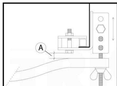
Make sure the whole system is in the right position, the wheel does not touch any vital parts and is well caught between the bottom and the bracket. Finally tighten the chassis mounting clamp bolts (torque 25Nm).
