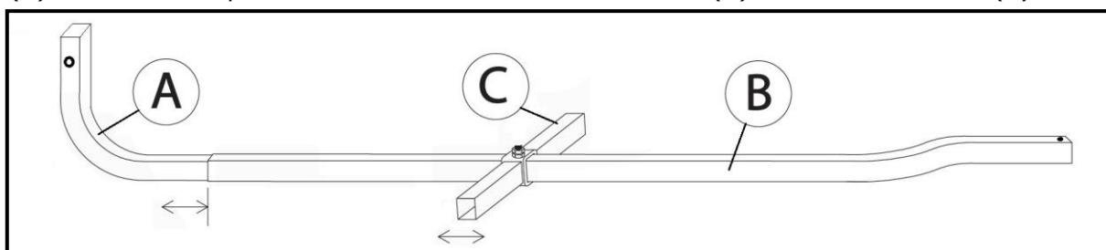
Place the assembled telescopic bracket under the caravan and attach the thinner tube (L -shape) to the left chassis bracket by the M10x60 bolt, 2 M10 washers and M10 locking nut (torque 5Nm). Because there are various spare wheel widths and chassis heights, three different heights are available. Make sure the spare wheel will finally be firmly fixes (caught) between the bracket and the caravan bottom. Possibly try first.
